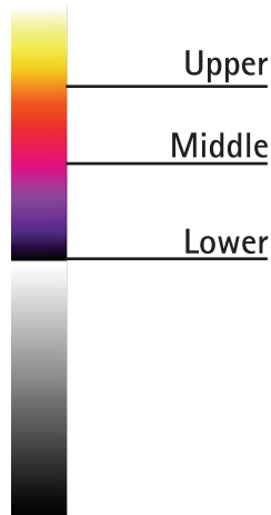
Figure 6. The Lower, Middle and Upper limits of an isothermal palette.
