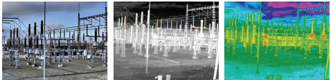
Figure 3: To the left an image from an Axis network camera, in the middle an image from an Axis thermal camera, and to the right an image from an Axis temperature alarm camera.
