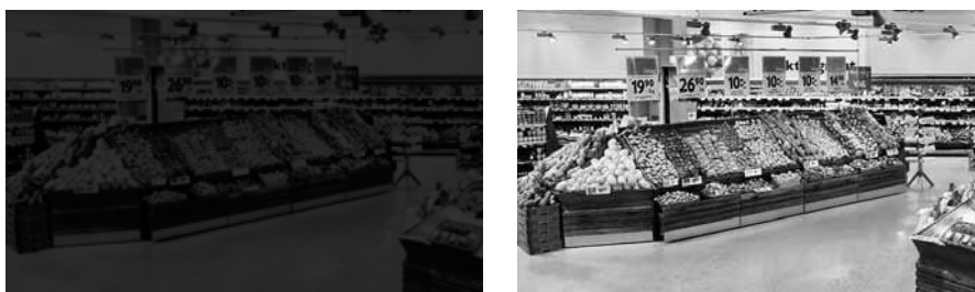
Figure 8 and 9: Same images as per figure 6 and 7, but taken with a Tele lens. To the left, the subject is not receiving enough IR illumination; while to the right the IR illumination is evenly distributed and the subject is not underexposed.
