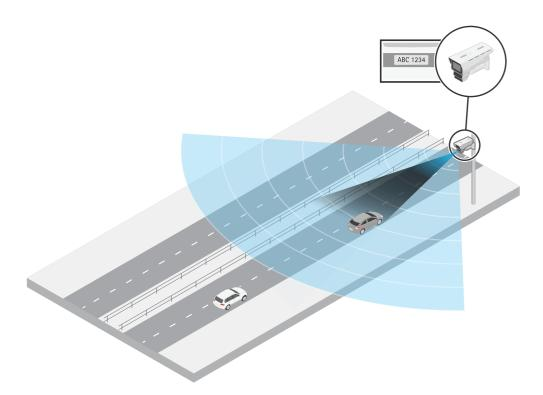
AXIS Q1686-DLE is mounted on a pole on the side of a highway, and measures the speed and captures the license plates of approaching vehicles.
