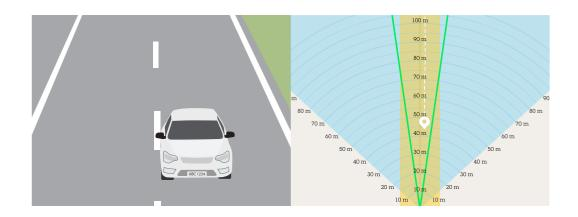
The camera view is illustrated on the left side, and the radar view with two added lanes in yellow on the right. The passing car is shown as a white track in the radar view, followed by a trail.
