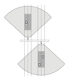
The same type of installation is possible if you want to capture license plates and the speed of vehicles that drive away from the radar-video fusion camera, instead of driving towards it.
