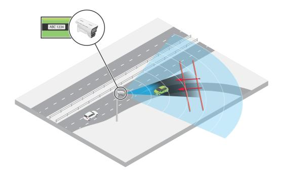
With this configuration, the radar detects vehicles and their speed when driving in the wrong direction. At the same time, the camera can provide visual identification and capture the license plates of the vehicles. With this setup it's possible to create rules for events, for example to trigger a recording when the vehicle crosses the lines, or trigger external lights that can warn the driver. Additionally, the license plate information can be processed on the server side.
