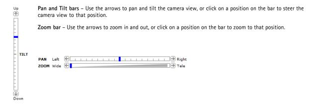
The PTZ controls can be disabled under PTZ > Advanced > Controls, see Controls, on page 22.
