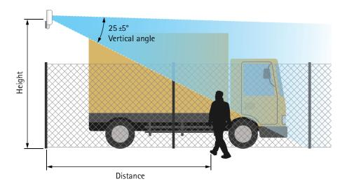
The following table shows the detection range at different mounting heights when detecting a 1.8 m (6 ft) tall person walking.
