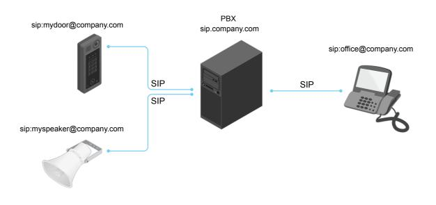
When you press the call button on an Axis door station, the call is forwarded through one or more PBXs to a SIP address either on the local IP network or over the internet.
