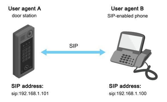
You can set up the Axis door station to call for example a SIP-enabled phone on the same network using a peer-to-peer SIP setup.
