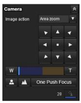
On this panel, you can control the pan/tilt/home position of the camera, adjust the zoom and switch focus mode (page 26). In addition, you can obtain authority to operate the camera when the exclusive control mode is on.
