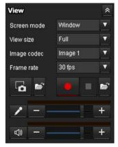
You can change the screen mode, size of the image, image codec mode and frame rate. Also, still images and movies can be saved (movie saving can also be stopped) from here. Microphone and audio output levels can be adjusted.
