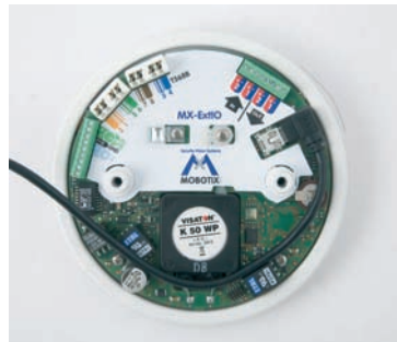
Insert USB plug Properly guide the cable
