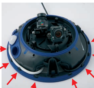
Lead cables properly through the cable guides
