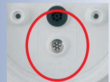
Mark for speaker inside the back
