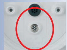
Mark for speaker inside the back
