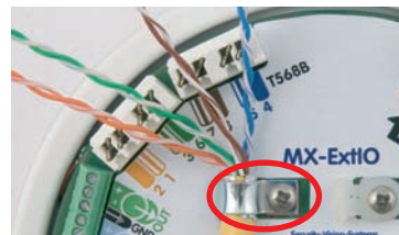
Lock cable in place with cable clamp
