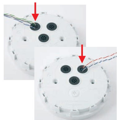
Push each wire through one of the openings of the 8-wire plug
