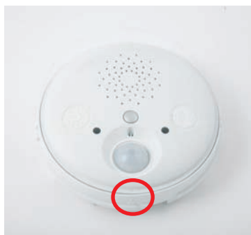
Assemble ExtIO housing Align arrows
