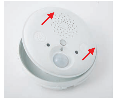
Remove the back of the housing
