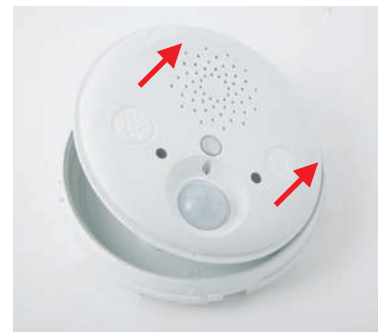
Remove the back of the housing
