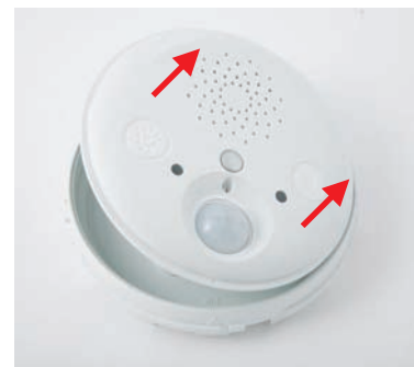
Remove the back of the housing
