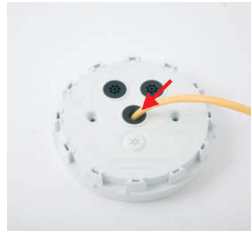
Insert cable into ExtIO's back and close off with rubber plug
