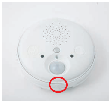
Assemble ExtIO housing Align arrows
