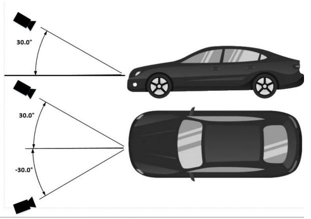
The image of the license plate should not tilt more than 5° horizontally. If the image is tilted more than 5°, we recommended to adjust the camera so that the license plate is displayed horizontally in the live stream.
