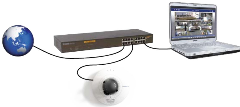
Fig. 16: Power supply using PoE switch according to PoE Plus (802.3at-2009).
