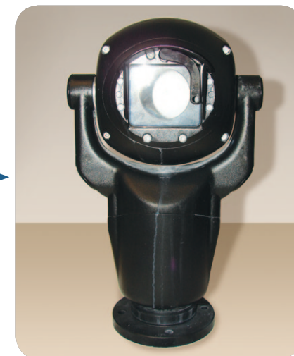
New MIC coating after 2000 hours salt spray
