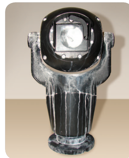
Older MIC coating after 2000 hours salt spray
