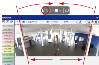
Section 3.5 provides more details and information on how the panorama and horizon correction works (correct distortion in the image and position horizontally)
