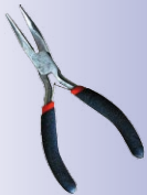
Pliers to break out cable guides
