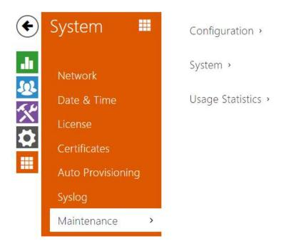
Use this menu to maintain your intercom configuration and firmware. You can back up and reset all parameters, update firmware and/or reset default settings here.
