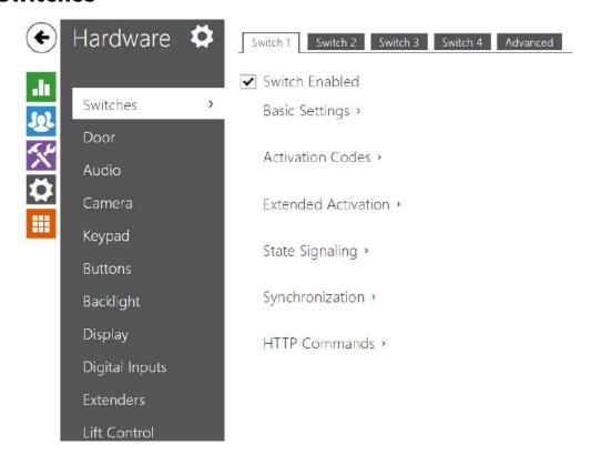
Switches provide a very flexible and efficient control of such intercom peripherals as electric door locks, lighting, additional ringing signalling, and so on. **2N LTE intercoms** allows you to configure up to 4 (depending on model types) independent all-purpose switches.
