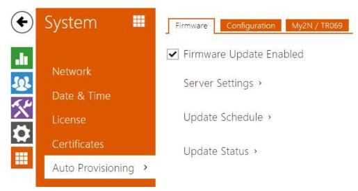
The **2N LTE intercoms** help you update firmware and configuration manually, or automatically from a storage on a TFTP/HTTP server selected by you according to predefined rules.
