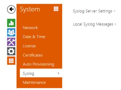
The **2N LTE intercoms** allow you to send system messages to the Syslog server including relevant information on the device states and processes for recording, analysis and audit. It is unnecessary to configure this service for common intercom operation.
