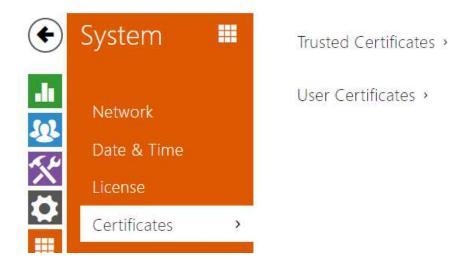
Some **2N LTE intercom** network services use the Transaction Layer Security (TLS) protocol for communication with other LAN devices to prevent third parties from monitoring and/or modifying the communication contents. Unilateral or bilateral authentication based on certificates and private keys is needed for establishing connections via TLS.
