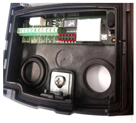
2) Insert the module of card reader into the shown connector.
