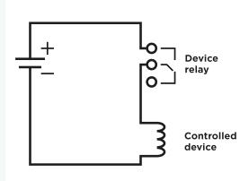
Wiring diagram for the controlled device electric circuit closing
