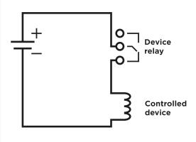
Wiring diagram for the controlled device's electric circuit opening
