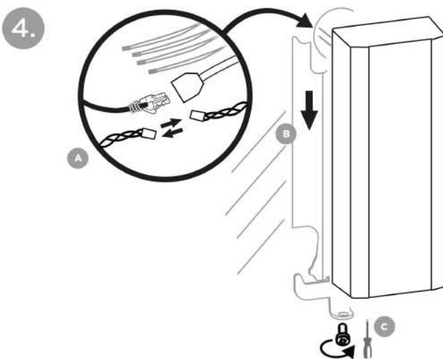
Interconnect the fed-out cables with the **2N Access Unit M** cabling. Put the device carefully on the installed holder from above downwards and fix its position on the holder carrying elements by tightening the screw from the bottom through the holder hole.
