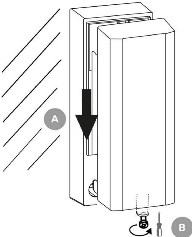
Insert the device on the holder by pulling it from top to bottom making sure that the holder stops drive under the screw heads on the device back side. When the device fits the holder carrying elements, fix the device position by tightening the screw to the device through the holder hole from the bottom.
