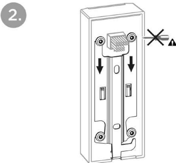
Pull the metal holder downwards to remove it from the device back side.
