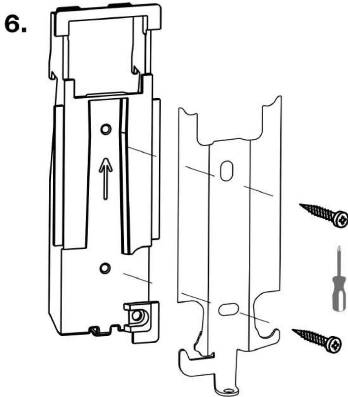
Fit the holder to the box cover using the included screws.
