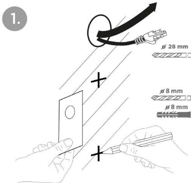
Use the drilling template shown on the device box to prepare holes of the required sizes for cabling and dowels on the selected place in the required height. Feed the cables out of the predrilled hole.
