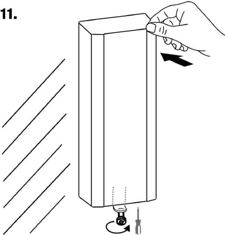
Replace the device into the vertical position and put on the holder. When the device fits the holder carrying elements, fix the device position by tightening the screw to the device through the holder hole from the bottom. Push the device upper part to fix the device in the final position.
