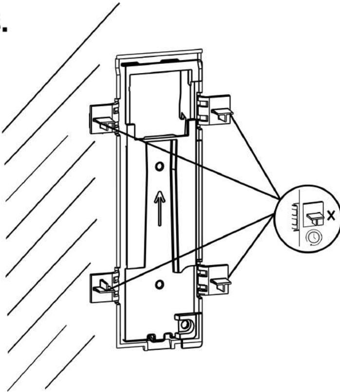
When the walling material has hardened, break off the box side stops.
