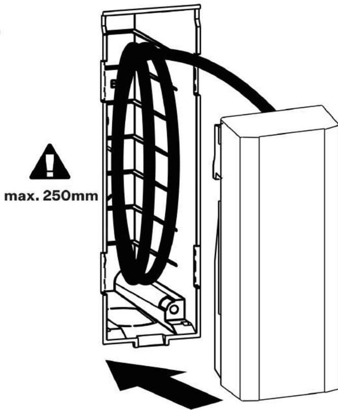
Insert the wires in the box keeping in mind that the maximum cable length is 250 mm.
