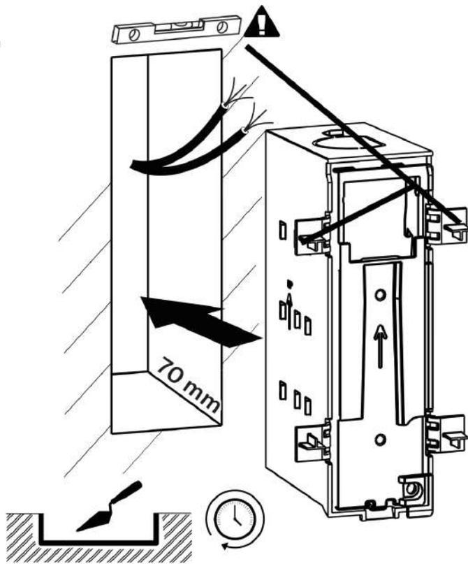
Replace the cover onto the box. The box works as a strut while walling in. If the box location is convenient, wall the box in.
