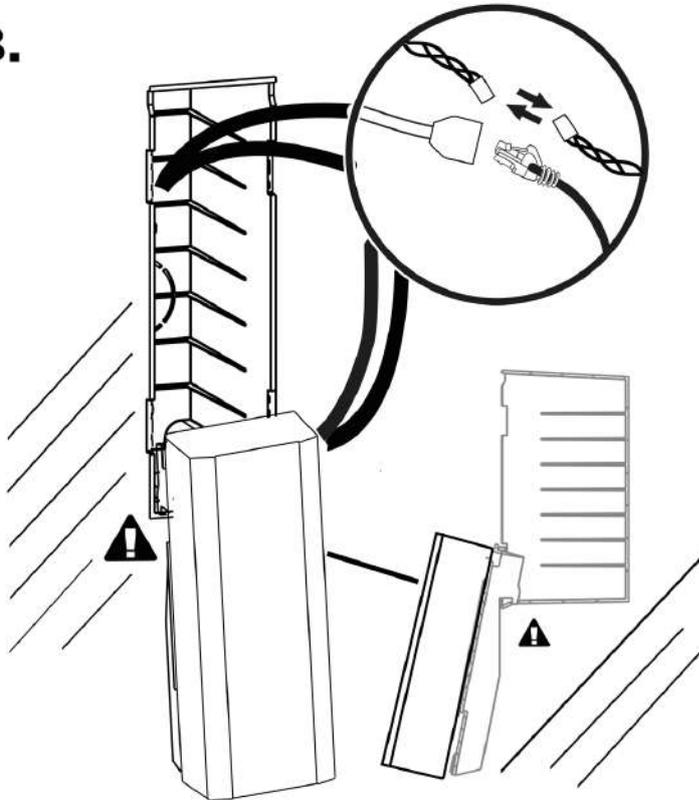
If you connect the device to installed cables, hang the device on the cover with the cover hooks into the box bottom holes. Connect the wires.
