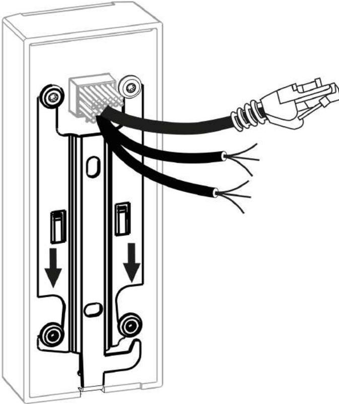
Pull the metal holder downwards on the device back side to remove it.
