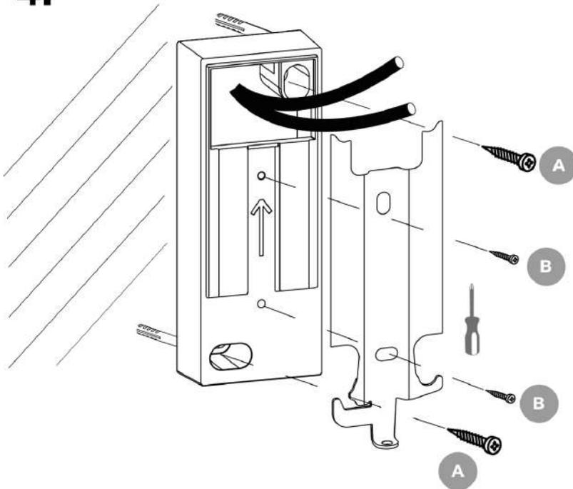
Anchor the backplate to the base using screws and dowels. Screw the metal holder to the backplate
