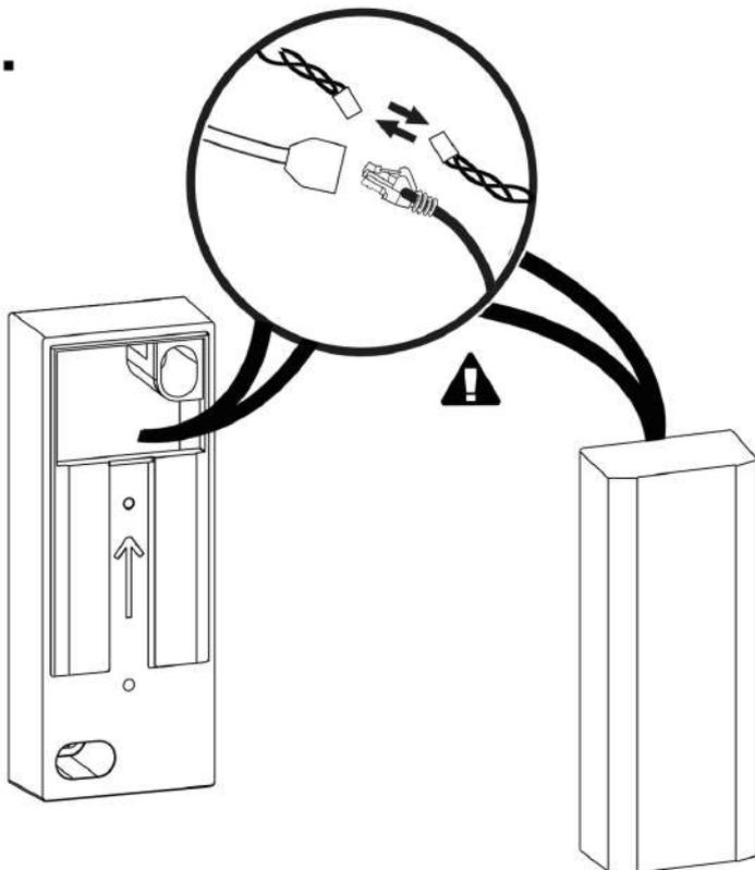
Put the cables in the backplate and put the backplate against the wall. If you connect the device to installed cables, connect the wires.
