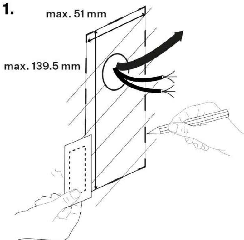
Make a hole of the size of 139.5 (h) × 51 (w) × 70 (d) mm for the mounting box installation. Remove the box cover and the cable installation blank.
