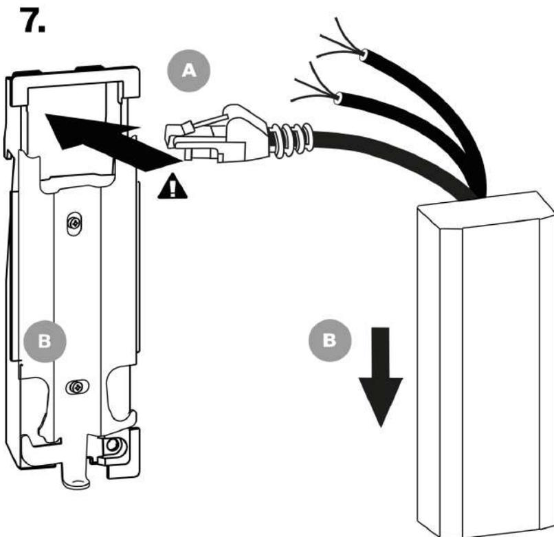
Pull the cables leading from the device through the cover hole. Press the holder screwed to the cover to the device and move it upwards carefully to make the holder stops drive under the screw heads on the device back side.
