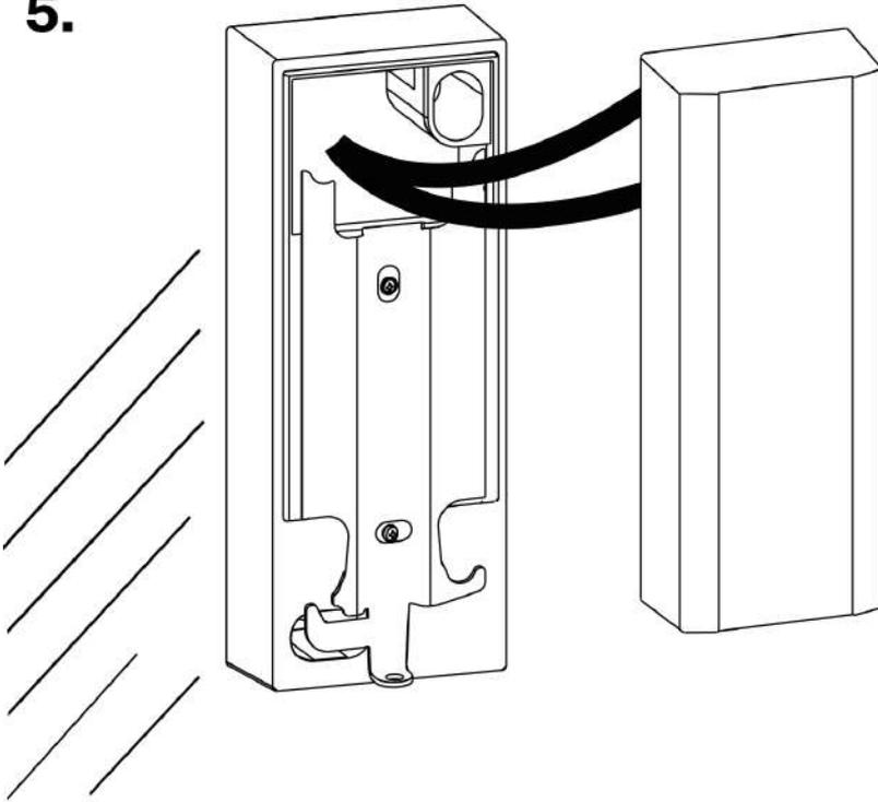
Put the device against the backplate and insert the remaining cables carefully in the backplate.
