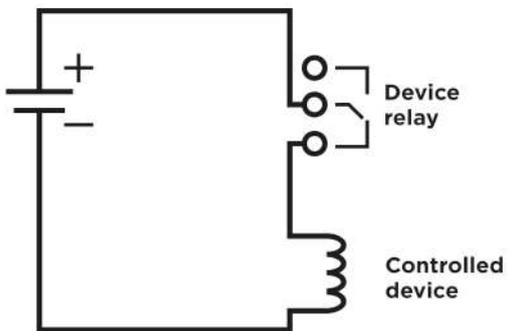
Wiring Diagram for controlled device's electric circuit opening
