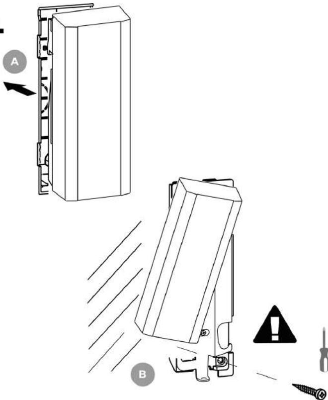
Insert the cover with the device in the box. Pull the device carefully upwards to release it from the holder. Turn the device bottom part by approx. 30° to the left along the wall without moving it away from the wall. Tighten the screw into the hole on the right-hand bottom part of the box to anchor the box cover.
