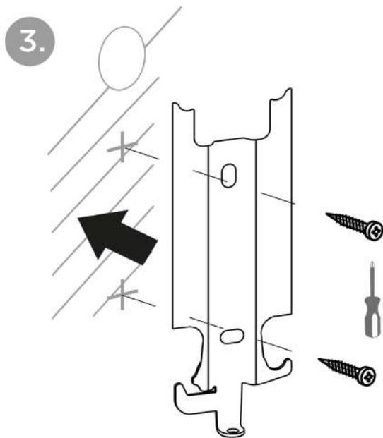
Then fit the holder through the dedicated holes using the screws enclosed.
